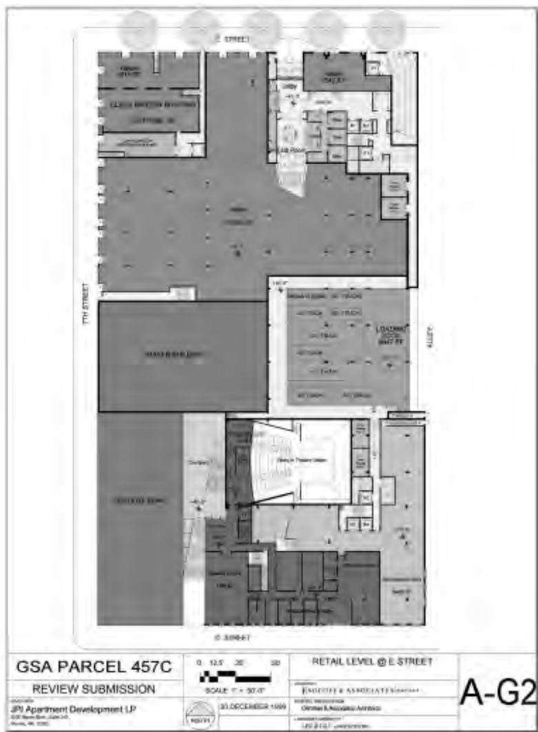
The E Street schematic retail level plan reveals JPI's proposed jigsaw of shops, theater, lobby, parking, and loading dock.
